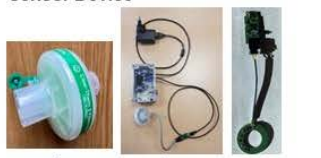
Figure 1. (A) Clear-Guard MIDI breathing filter with Luer port; (B) Sensor device adopted for use in mechanical lung ventilation machine; embedded in the breathing filter, a sensor signal registration device (Raspberry Pi), and a power adapter; (C) Sensor board connected to a micro-USB cable.
