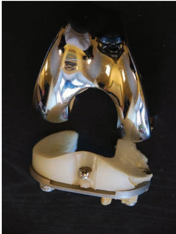
Fig 9. Removed endoprosthesis due to polyethylene wear.
