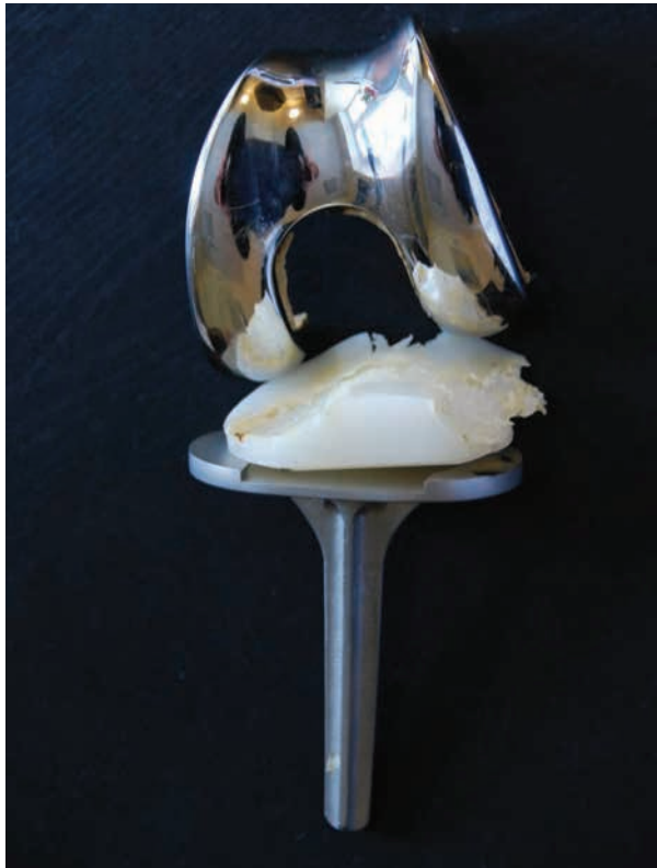
Fig 10. Removed endoprosthesis due to polyethylene wear.
