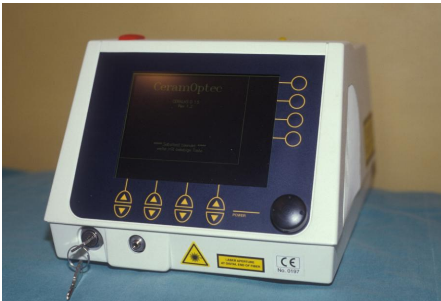
Figure 1. Compact size air-cooled diode laser Ceralas D15
