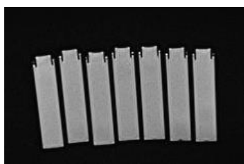
Fig. 8. T2 MR image of MAGAT gels with admixed small amount of AgNO 3 irradiated to different doses.
