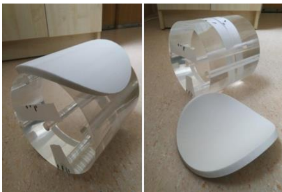
Fig. 3. Standard CT PMMA head phantom and 3D printed polyactic acid plastic (PLA) bolus.
