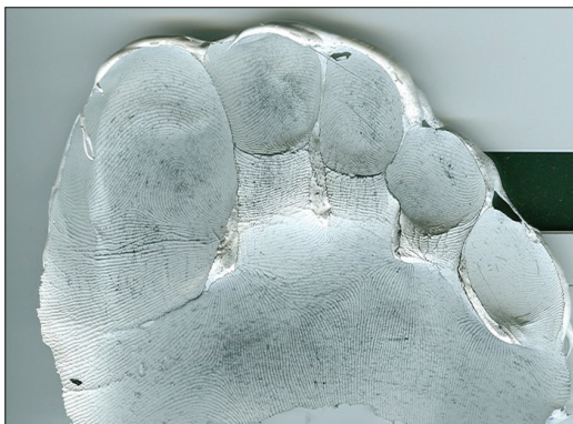
Figure 2. Toes of the right foot recorded with white Microsil ® , lightly tinted with soot powder
