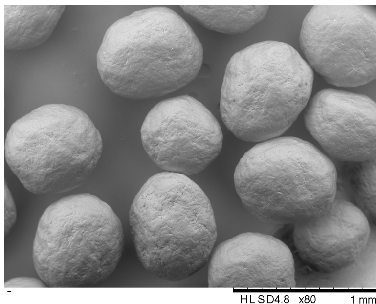
Figure 3. SEM of MCC spheres (D10% = 563 μm, D50% = 651 μm, and D90% = 696 μm).
