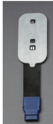
Figure 2. INVOS sensor with one light diode and two light detectors (picture taken from The INVOS Cerebral/Somatic Oximeter Operations Manual, Covidien 2010).
