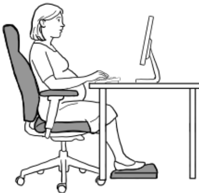
Figure 4.2. Ergonomic workstation setup for a pregnant nurse, including reclined seating, desk height adjustment, and footrest. Adapted from Anderson & Johnson (2004).
